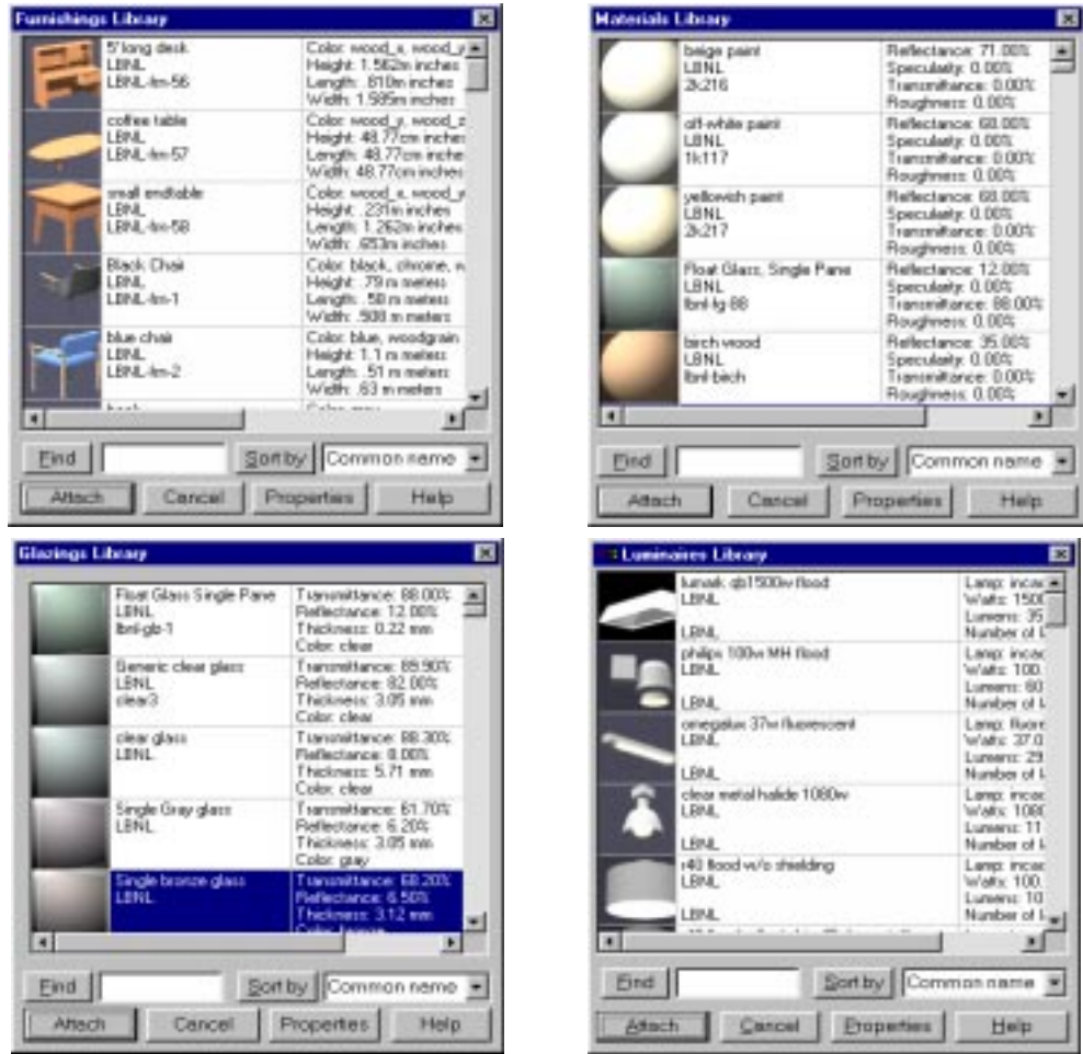
FIGURE 1 GRAPHICAL USER INTERFACE ALLOWS DESKTOP RADIANCE USERS TO SELECT MATERIALS, GLAZINGS, LUMINAIRES AND FURNITURE FROM CORRESPONDING LIBRARIES.
